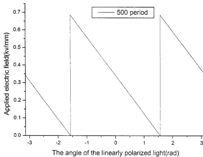
Fig. 4 Relations between applied electric field and the polarization angle of the light
