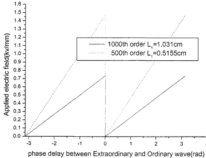
Fig.2 the relationship between the applied electric field and the phase delay of the extraordinary and ordinary wave
