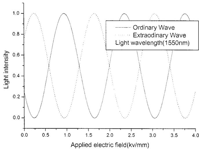
Fig.3 Power exchange relations between the extraordinary and the ordinary wave when the phase matching condition is satisfied ( $\Delta\beta = 0$ )
