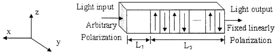
Fig 1. The basic structure of an electric polarization controller, X, Y, and Z represent the principal axes of the original index ellipsoid. The arrows inside the PPLN indicate the spontaneous polarization directions.
