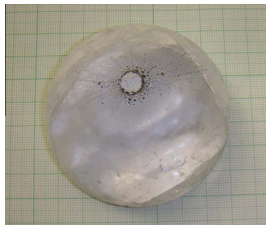
Fig. 1. \text{BaMgF}_4 crystal grown by temperature gradient technique.
