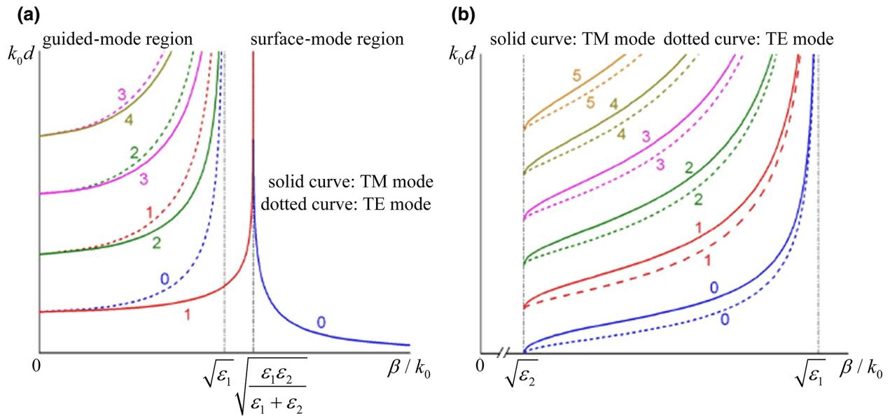
FIG. 2. Dispersion curves of (a) the MCOR and (b) a symmetrical dielectric waveguide.
